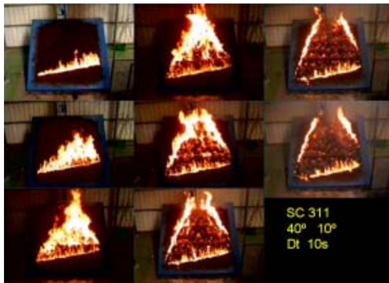
Figure 1. Laboratory experiment of a non-horizontal fire front spreading on a 40° slope.
